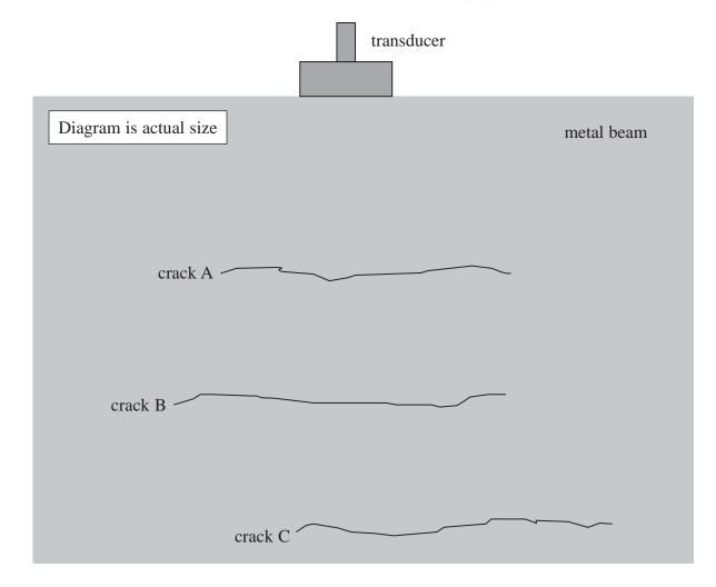
The transducer detects a returning pulse from each crack.
